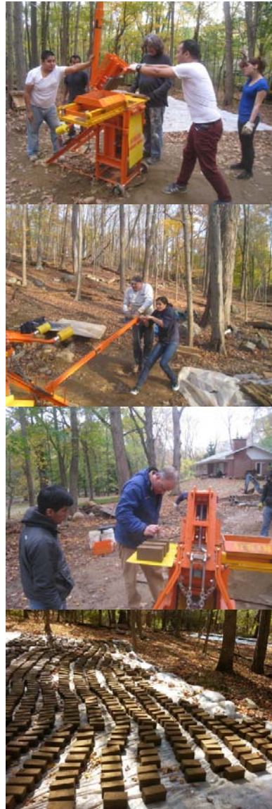
From top: Simal closing the top of the Aurom 3000; Michael and daughter pulling down the level; bricks curing; Ashok testing a run of bricks; freshly compressed books curing.
