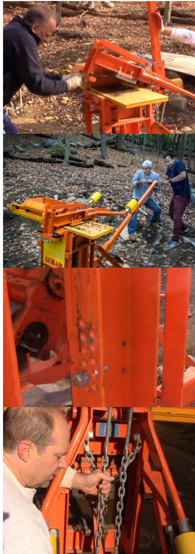
From top: Closing the top of the machine; Pulling down the lever (photo by Philip Jensen-Carter); the location of two bolts determine the depth of the compression; the two chains in the front must be tighter than the "V" chain (behind the hand) for the machine to pop the top at the right time.
