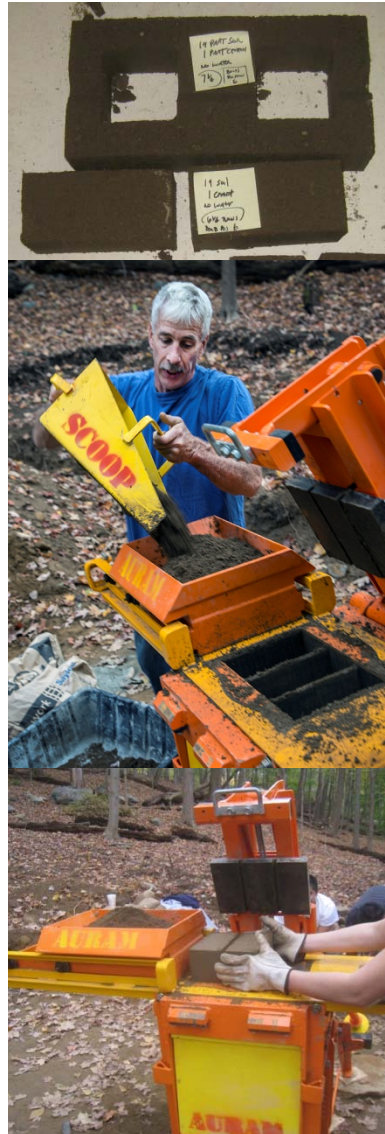
From above: The hollow brick above was too hard to handle before it cured so we opted for the smaller solid bricks; Filling the hopper (photo by Philip Jensen Carter); removing the bricks
