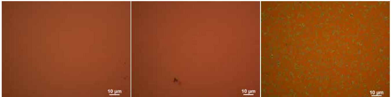
Figure 2. The samples. Left: Sample 1 (Al 600 °C/Si 600 °C). Middle: Sample 2 (Al 600 °C/Si 600 °C). Right: Sample 3 (Al 600 °C/Si 650 °C).
